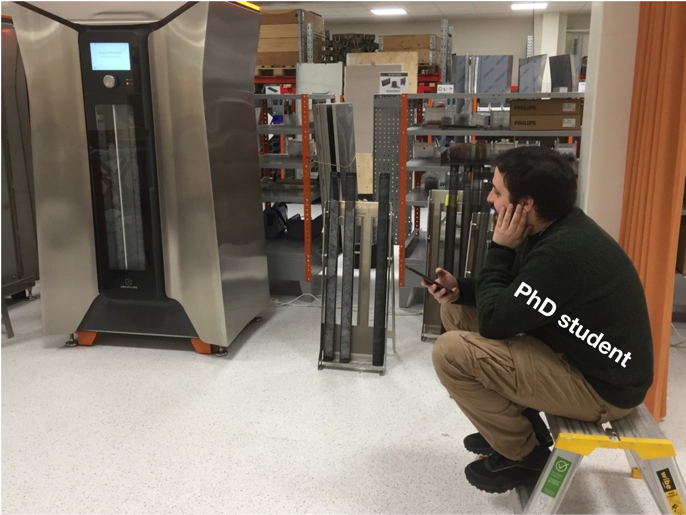
Orexlore GeoCore X10 XCT-XRF drill core scanner
